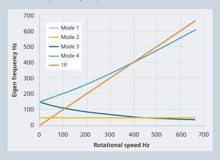
In a rotor dynamics analysis, the system's critical speed is particularly important. The critical speed corresponds to a rotation speed that is equal to the modal frequency. Because the critical speed is the speed at which the system can become unstable, engineers must be able to accurately predict those speeds as well as detect possible resonance problems in an analysis.
